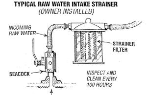
**NOTE:** The external thru-hull opening should be of the flush type with a clear opening. No perforated or slot type external opening. Let all the filtering be accomplished on the inside of the hull where there is easy access to the strainer.
