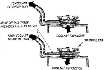
**NOTE:** Periodically check the condition of the pressure cap. Ensure that the upper and lower rubber seals are in good condition and check that the vacuum valve opens and closes tightly. Carry a spare cap.
