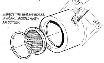
**WARNING:** The generator should never be started/operated without the air screen/flame arrester properly installed.
