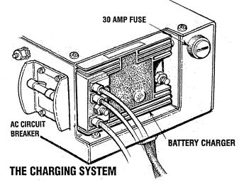
The battery charger is an encapsulated, solid-state unit that supplies a DC charging voltage to the generator's starting battery while the generator is operating.
